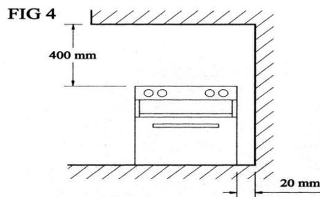
Ensure that no obstruction to the units air flow is permitted at the base, sides or back. Obstruction of the air flow can cause inefficient combustion in the oven.
