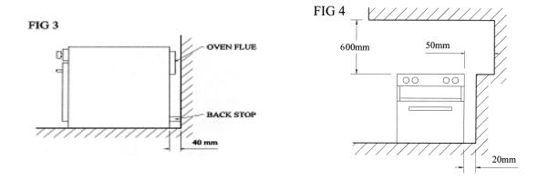
There should be no obstruction above the hob burners for a minimum height of 600 mm (24"). (FIG 4)
