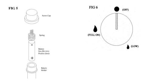
Some models are fitted with a spark ignition system. These use a  $1 \times R6$  (AA) battery. The spark system will only work if the battery is correctly inserted into the holder (Fig 5). The battery holder is located to the bottom right hand side of the cooker. Lighting a burner is as described above. The spark to light the burner is applied by pressing the switch on the front right hand side of the facia panel.
